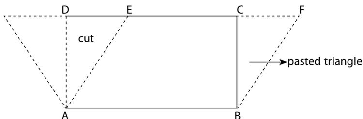
Cut the triangle ADE and paste it on the other side with BC to form triangle BCF.
