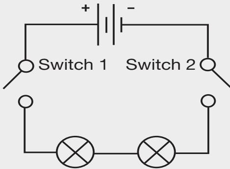
3. What should be done in the circuit so both the lamps will be lightened?
