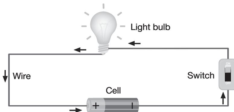
2. Maria connected different materials to the circuit to check if the bulb glows. If the bulb glows it means that the material can conduct electricity or it is a conductor.
