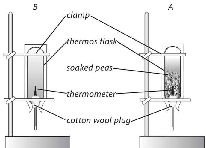
Turn both flasks upside down and fix them in retort stands as shown. Make sure that the thermometer in flask A is in the middle of the seeds.
