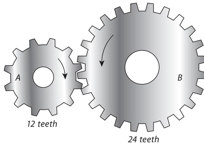
Count the number of teeth in the two gear wheels of the food mixer or drill and calculate their speeds.
