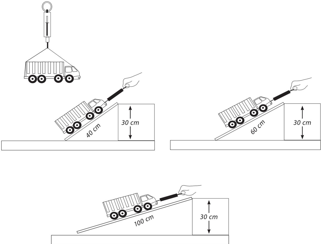
2. Use the newton meter and some string to determine the force (resistance =  $R$ ) needed to lift the truck and its load vertically.
