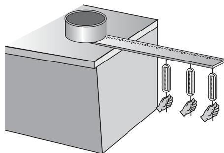
Now put the 20 cm mark at the edge of the desk and push down, or pull down with the force meter. Measure how far you have to move the ruler to lift the load 8 cm.
