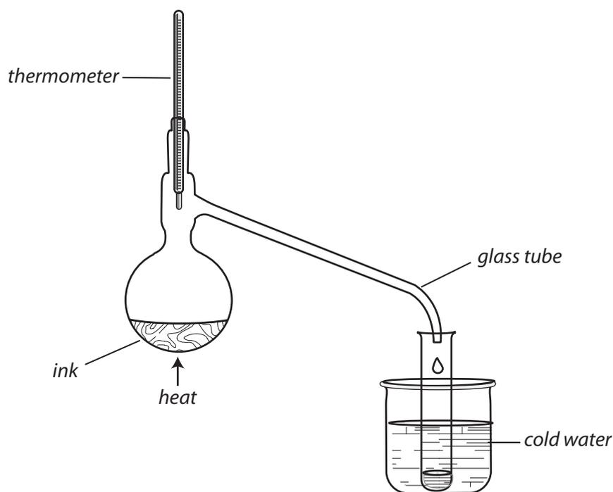
3. Using the Bunsen burner, heat the coloured water gently. If you heat the water strongly steam may shoot up the delivery tube.
