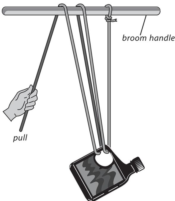
4. Tie one end of the rope to the broom handle. Loop the rope through the bottle handle, and lift by the free end of the rope with the weight in the middle. This is equivalent to a movable pulley.
