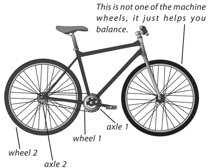
Using chalk and a meter rule or tape measure, find out how far the cycle moves for one turn of the pedal. Record your results:
